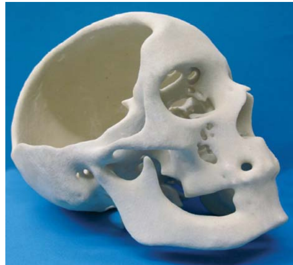
Figure 5. Image of a polymer-based custom-made skull model with a large defect obtained using a 3D printer (ZPrinter®).
